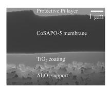
**Microwaving plates**: A facile method was developed for the fabrication of preferentially c-oriented cobalt-substituted silicoaluminophosphate-5 (CoSAPO-5) membranes on porous alumina supports. In situ microwave growth using a slip-coated  $TiO_2$  layer on the support surface resulted in an oriented CoSAPO-5 crystal layer, which was evolved into a defect-free membrane by improving crystalline intergrowth through secondary hydrothermal microwave growth.
